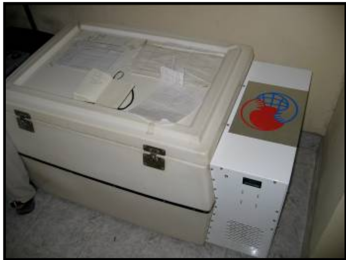
Figure 1: WHO installed solar powered vaccine refrigerator has worked well for two years. A smaller solar system has worked for 6 years powering the radio.
