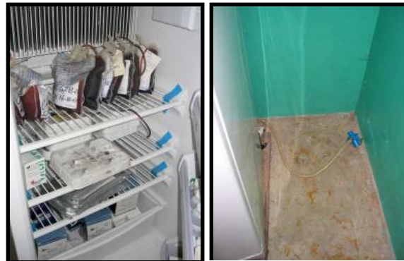
Figure 1: The contents of this refrigerator were at room temperature because the propane had run out.
