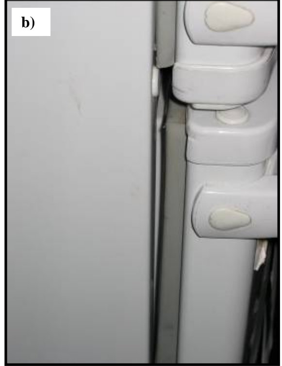
Figure 3: a) CDC provided blood lab refrigerator not connected to gas or electric power b) gasket on refrigerator faulty, c) contents of refrigerator at room temperature, d) temperature log out of date, and e) blood bank refrigerator not in use because of insufficient power.
