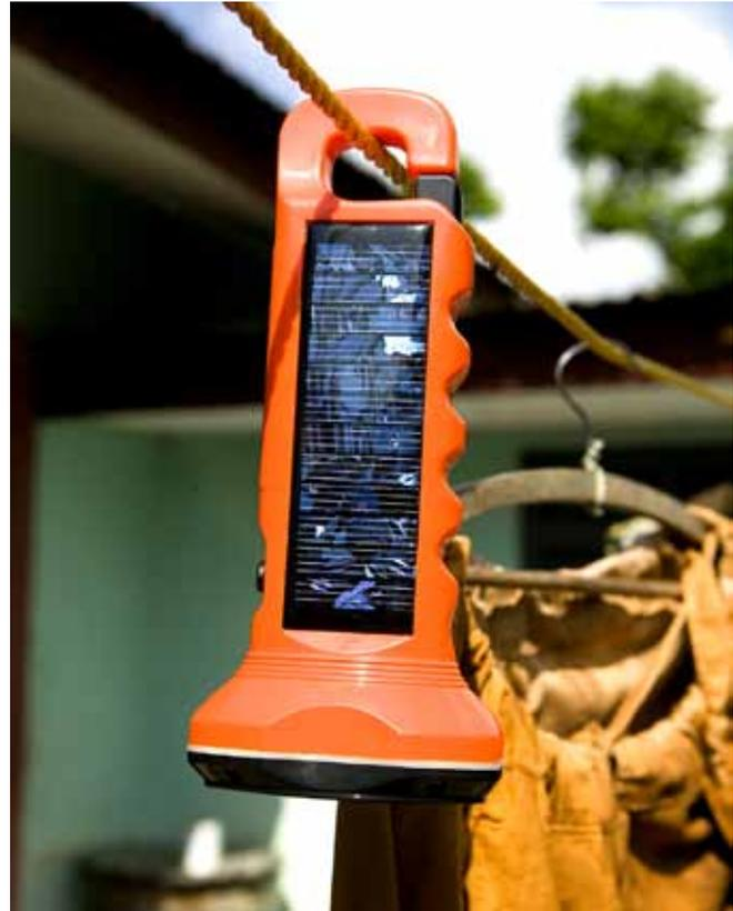
THIS BOGO FLASHLIGHT HANGS OUTSIDE ON A CLOTHESLINE DURING THE DAY TO CHARGE IN THE SUN. THE FLASHLIGHT PROVIDES USERS WITH SIX TO EIGHT HOURS OF LIGHT WHEN FULLY CHARGED. PHOTO | COURTESY OF SVEN WIEDERHOLT
