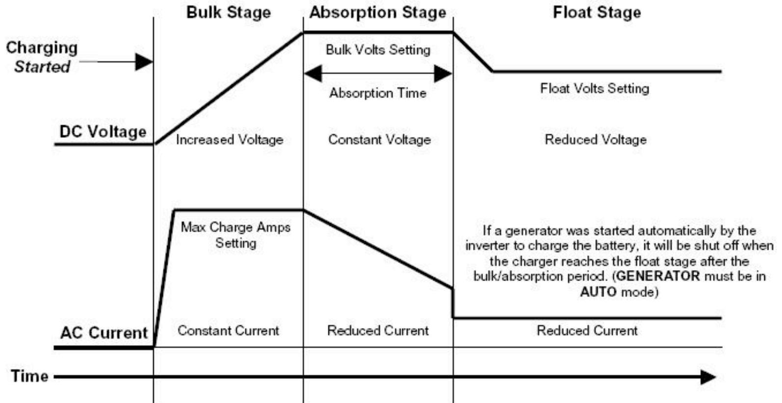
Figure 21, Three-Stage Battery Charging
